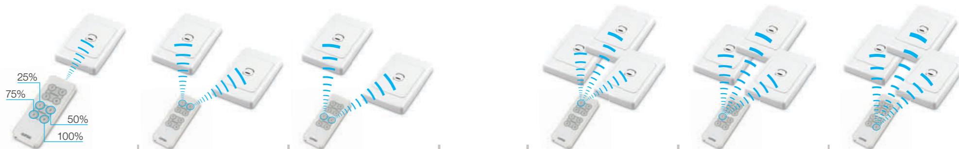
Dimming one light, with four different preset scenes
