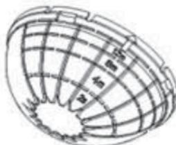
Engraving indicates the approx detection range of each section
