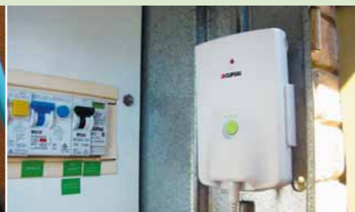
2 Plug into the Transmitter Unit which relays power use to the Receiver Unit.
